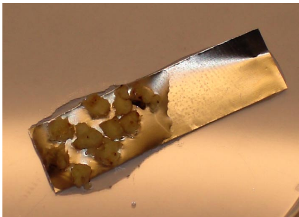
Figure 13. Meristem clumps in a droplet of PVS2 solution (of about 15 \mu l) on a strip of aluminium foil (5x20 mm).
